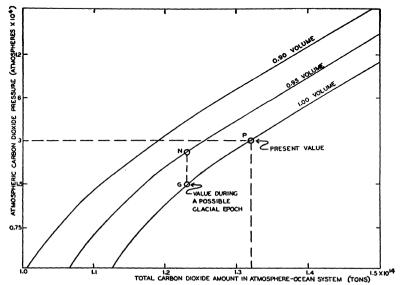
The equilibrium pressure of carbon dioxide in the atmosphere as a function of the total amount of carbon dioxide in the atmosphere-ocean system. Curves are shown when the oceans have 0.90, 0.95 and 1.00 times their present volume. The present value for these quantities is indicated by the letter "P." The line between "G" and "N" represents a possible oscillation of the climate during a glacial period.
